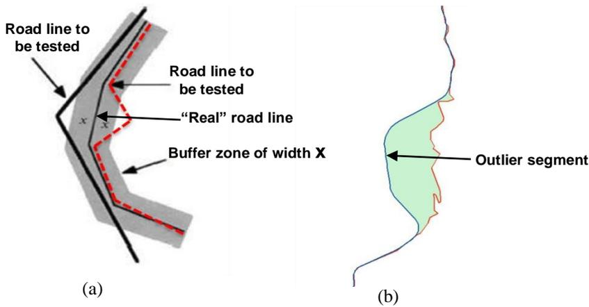
Figure 8. Weaknesses of (a) buffer method and (b) average distance method
