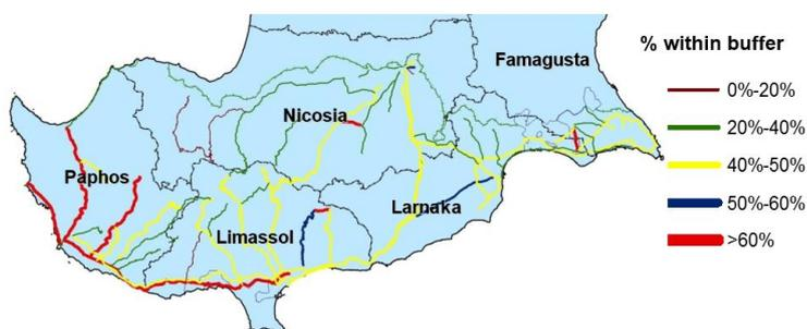
Figure 6. The spatial distribution of positional accuracy (for a 3m buffer) and the relevant classification of roads
