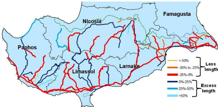
Figure 9. Length completeness per road with less or excess length.
